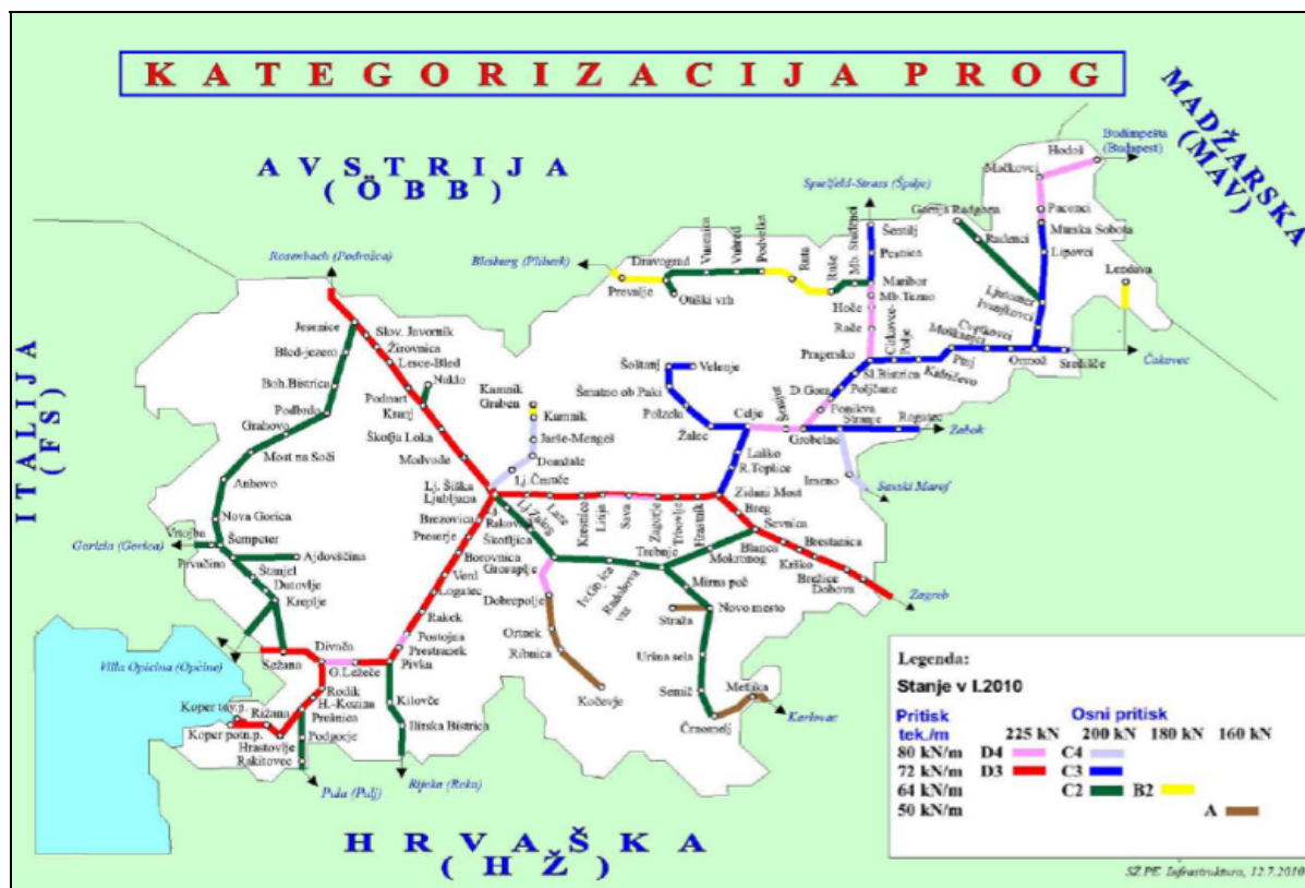
Figure 61 Load-bearing capacity of railway tracks
