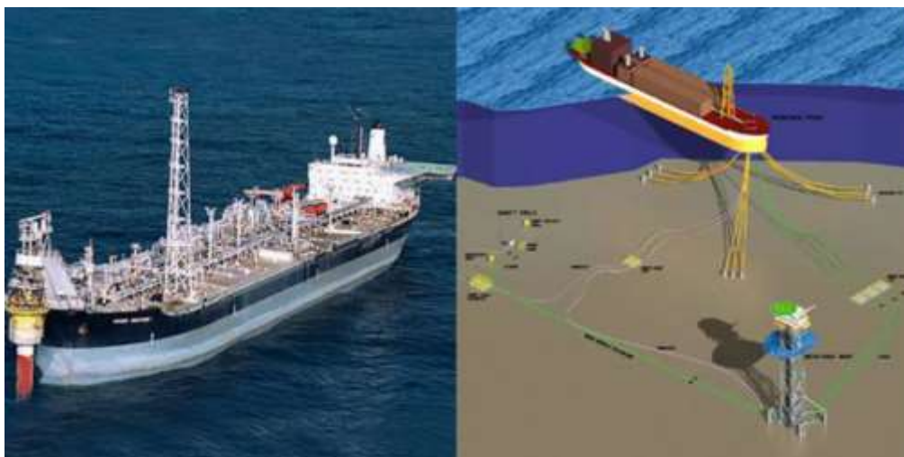
Figure 1.13 Floating production, storage and offloading systems for hydrocarbons (Source: https://www.rigzone.com/training/insight.asp?insight_id=299&c_id=12 )
