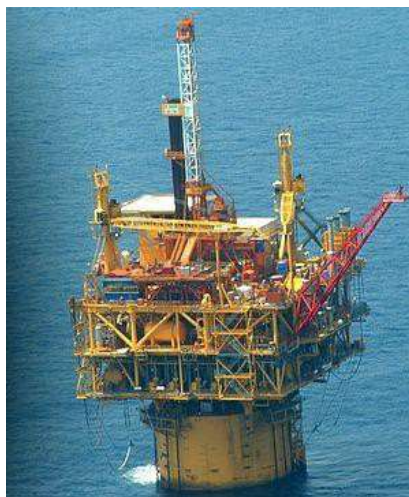
Figure 1.10 Floating spar platform (Source: http://en.wikipedia.org/wiki/Spar_(platform) )
