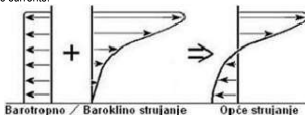
Figure 3.12 Schematic overview of the breakdown of current into its components
