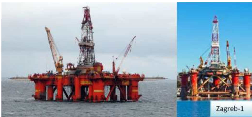
Figure 1.11 Semi-submersible platforms (Source: http://en.wikipedia.org/wiki/Semi-submersible )
