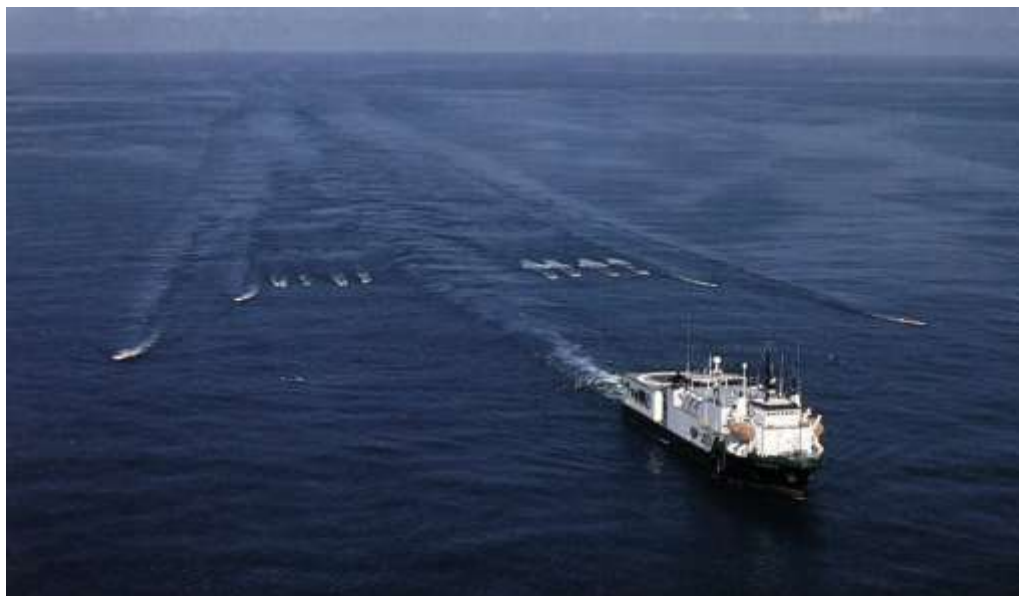
Figure 1.17 3D seismic imaging with 4 streamer lines and a number of airguns (Source: Dragoset, 2005)
