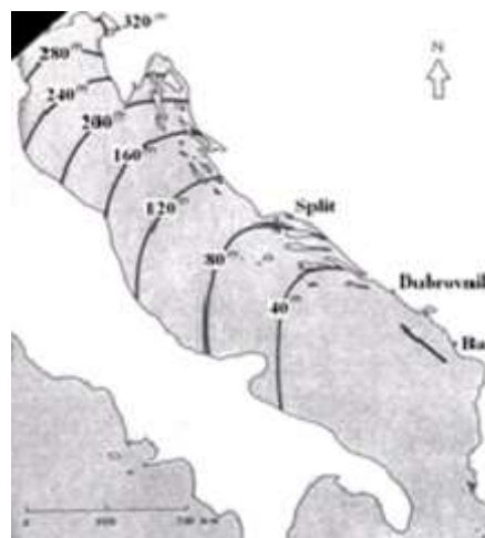
Figure 3.30 Motion of an earthquake wave in the Adriatic Sea. 1979 earthquake in the seas of the Montenegrin coast. Time calculation of the arrival of the wave front, in minutes (Orlić, 1984)
