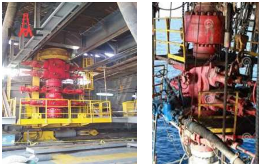
Image 1.23 Blowout preventer – BOP (Source: http://www.drilltech.cn/ufile/201465103760572.jpg )
