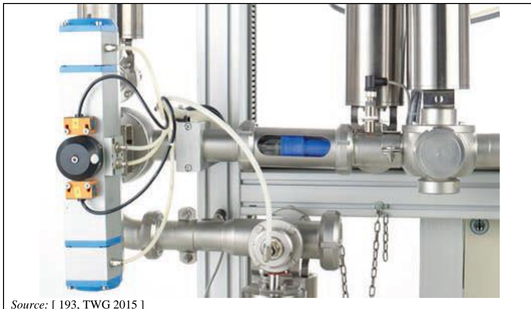
Figure 2.11: Pigging system
