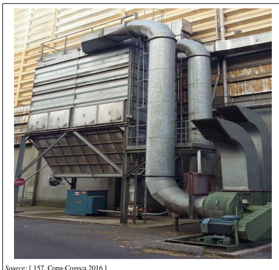
Figure 2.43: Picture of an industrial bag filter
