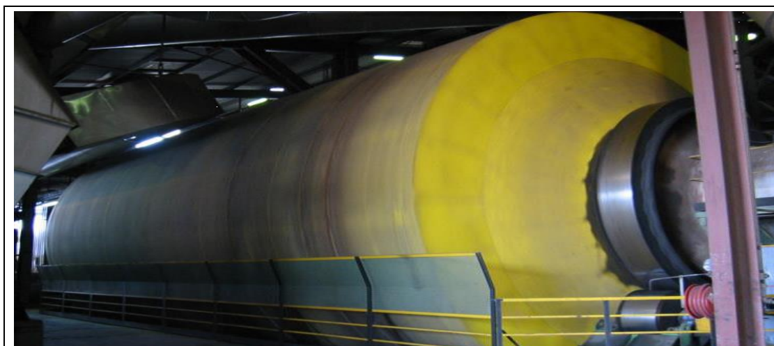
Figure 3.9: Three-pass drying drum
