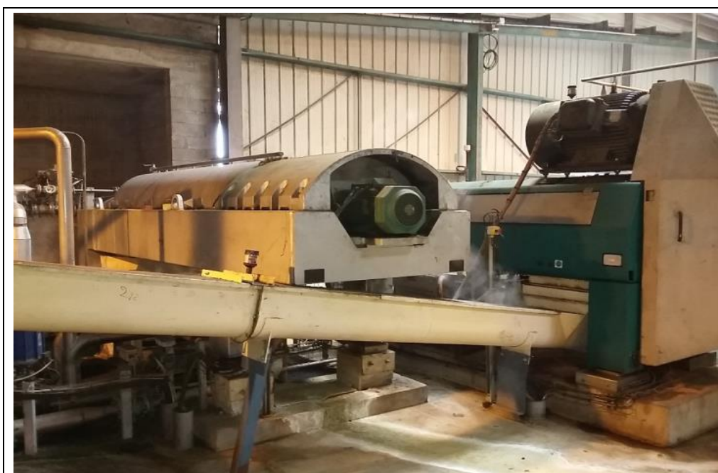
Figure 3.10: Centrifuge system in a dehydration site
